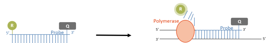
Figure 1. Principle design of dual-labeled probes. The primer is elongated by the polymerase, and the probe binds to the specific DNA template. Hydrolysis releases the reporter from the probe/target hybrid, causing an increase in fluorescence. The measured fluorescence is directly proportional to the amount of target DNA.
